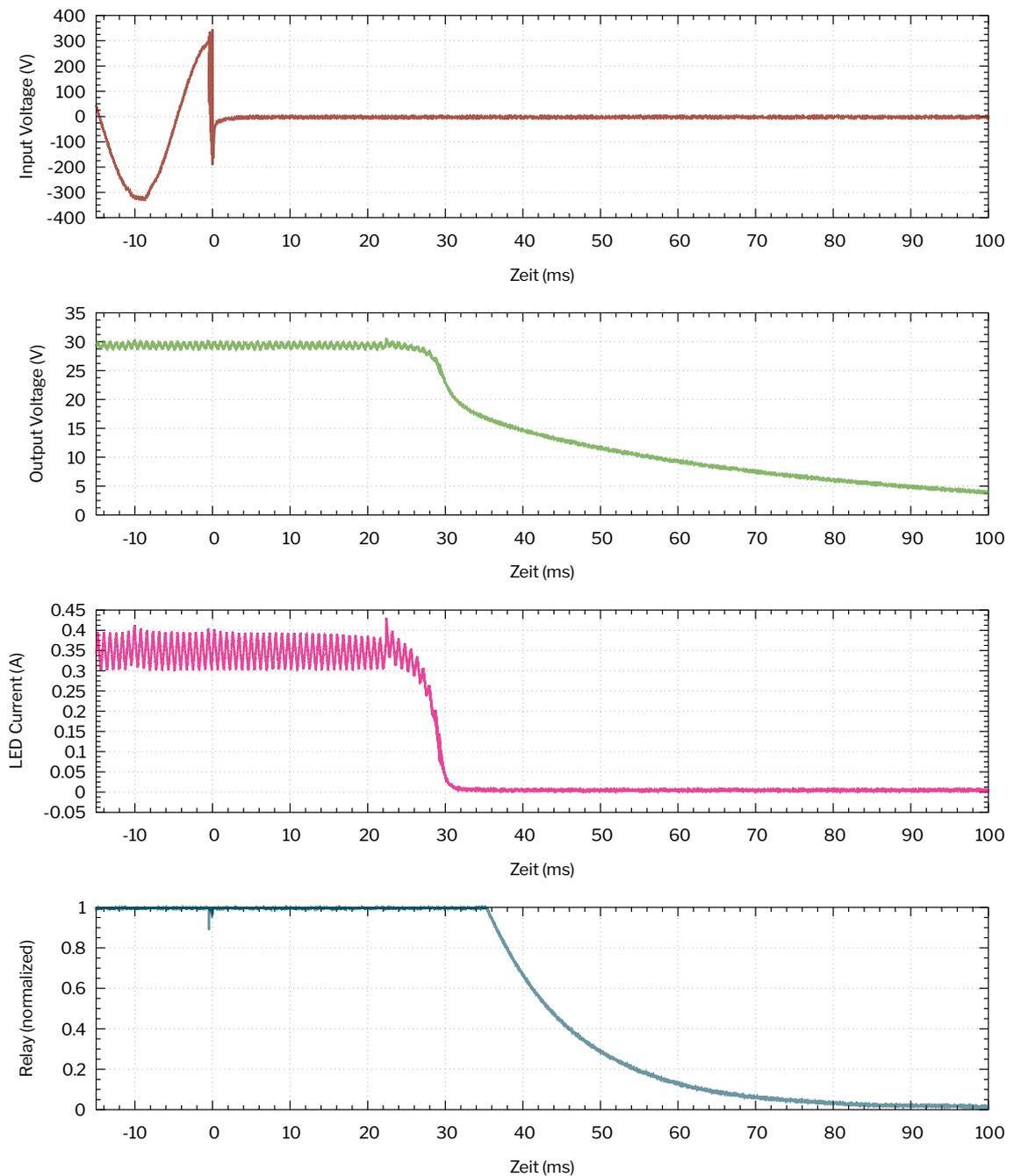
Figure 11: ACL230's AC turnff (disconnection) is shown.
