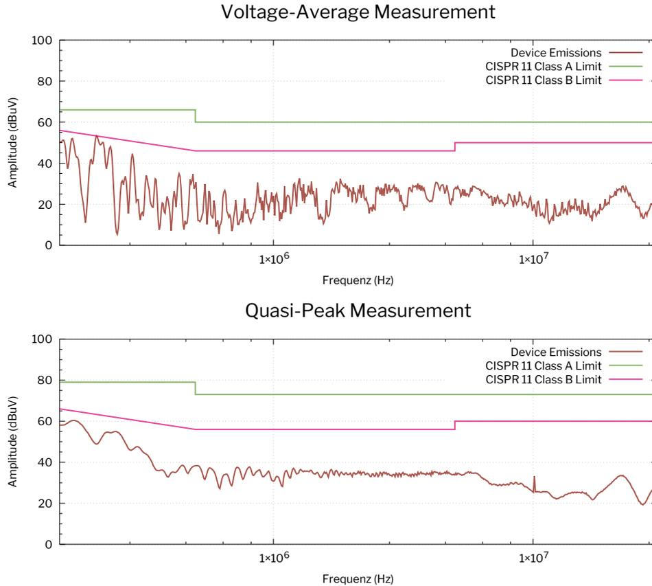
Figure 13: ACL230input (AC) line emissions.
