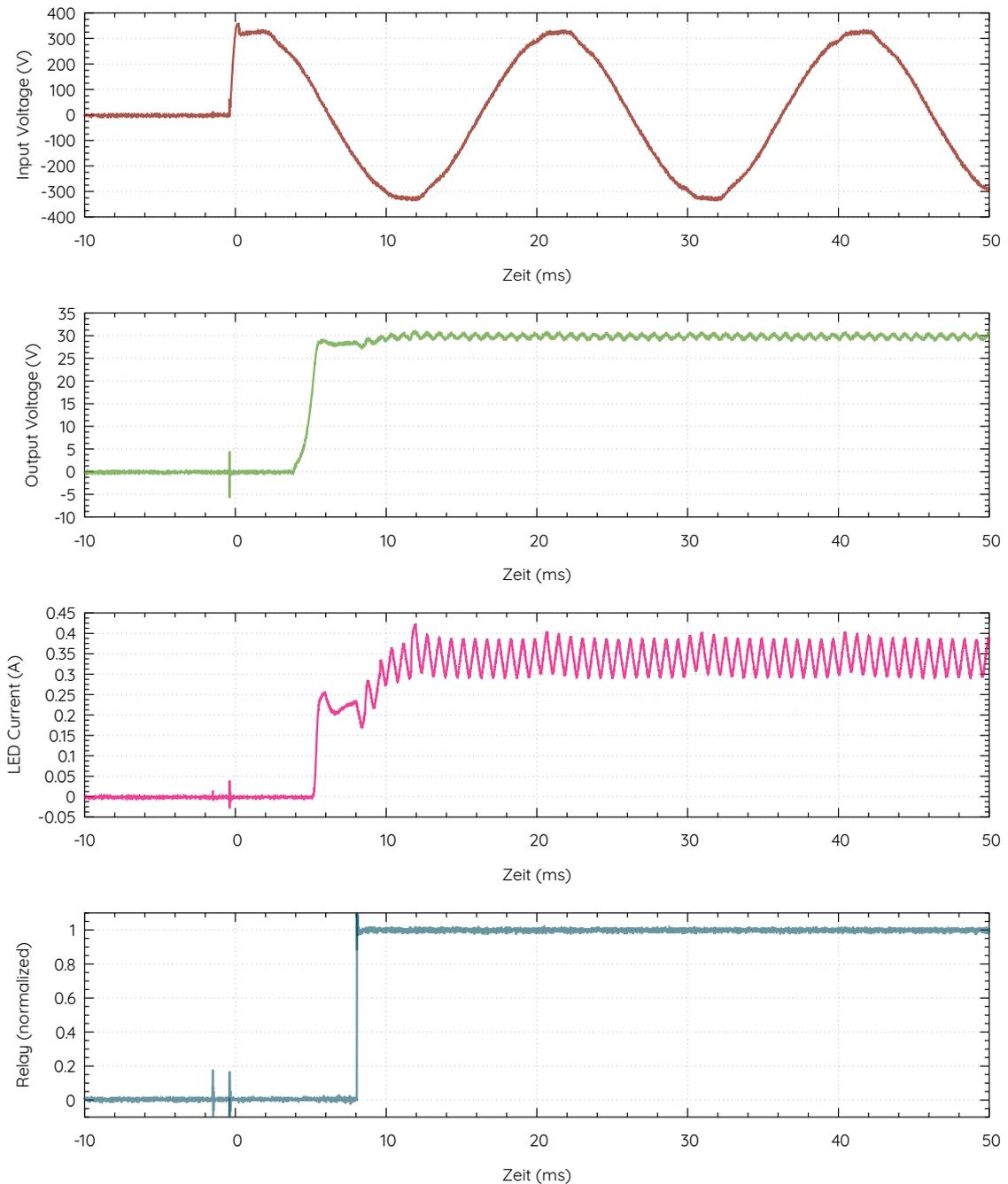
Figure 10: ACL230's AC turnon (connection) is shown.
